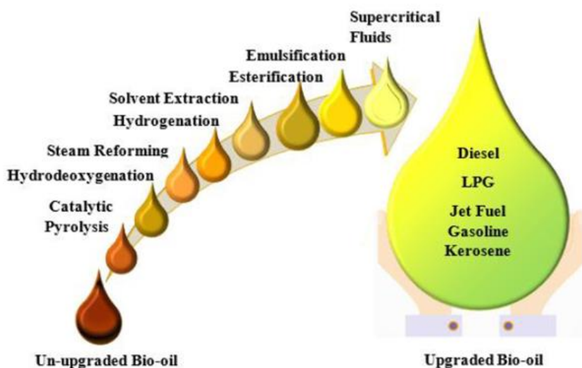
Figure 4. Different processes for bio-oil valorization. Adapted from [9].
