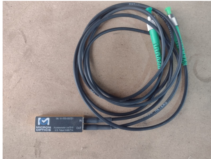
Figure 3.7 – Optical accelerometer based on Fabry Perot, model os7510.
