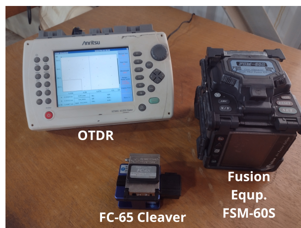
Figure 4.6 – Fiber optic welding equipment.
