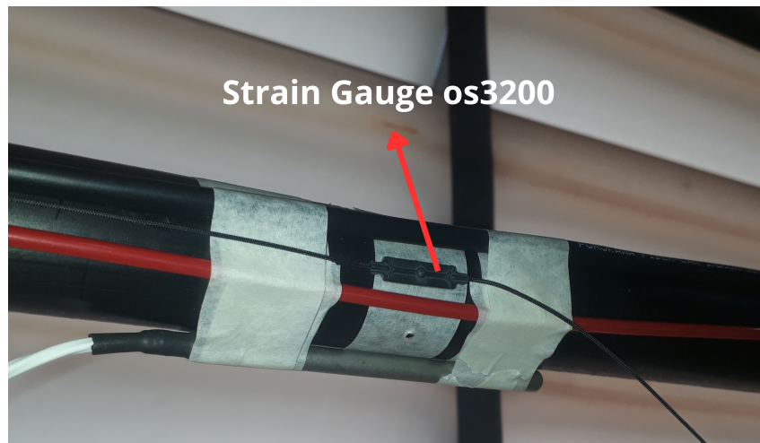
Figure 5.19 – Strain Gauge os3200 installed in the pipe close to the leak region.
