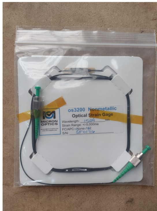
Figure 3.6 – Optical Strain gauge based on FBG, model os3200.
