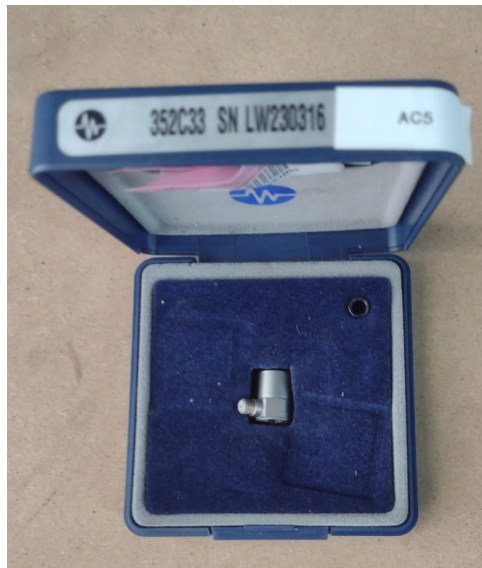
Figure 5.15 – Piezoelectric accelerometer model 352C33 in its box.
