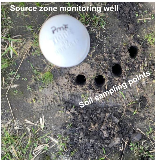
**Figure S3.** Example of source zone monitoring well and soil sampling points.
