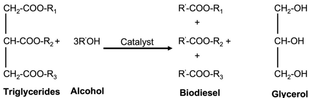
**Figure 4.** Triglycerides transesterification process to obtain Biodiesel
