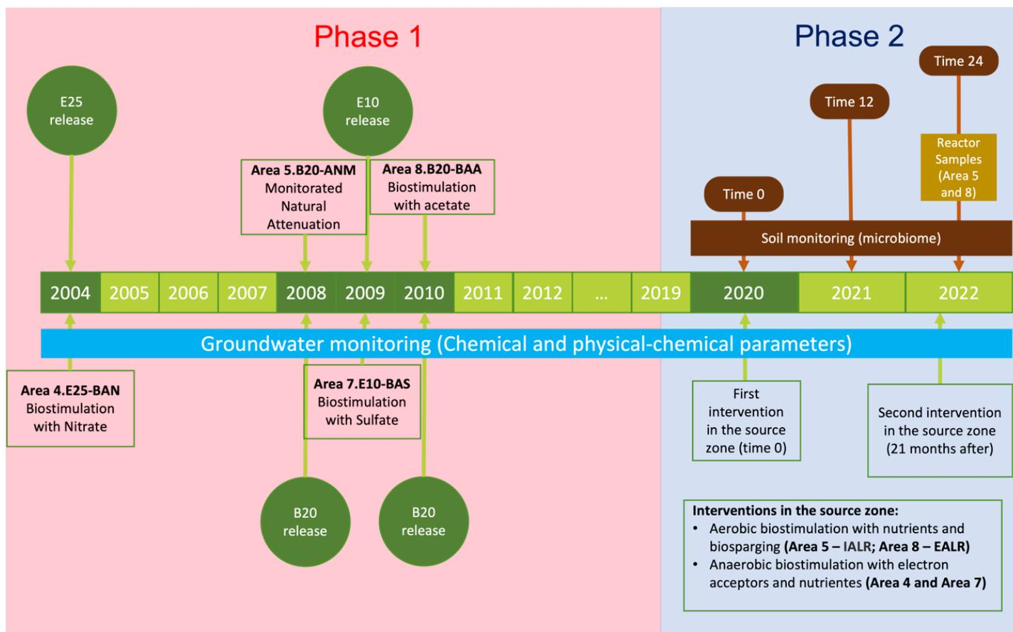
**Figure S2.** Timeline of the fuel releases and bioremediation treatments and details of the experimental areas.
