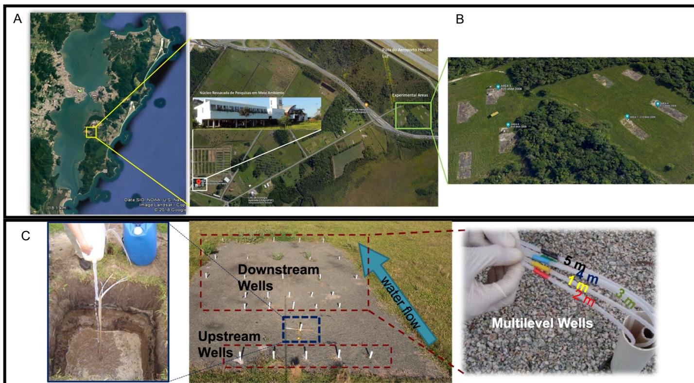
**Figure S1.** (A) Satellite view of the Florianópolis Island and the Ressacada Experimental Farm. (B) Satellite view of the experimental areas configuration. (C) From the left to the right: Fuels release, spatial monitoring wells distribution along water flow direction and identification of monitoring levels. Square dashed in blue indicates the source well
