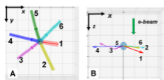
Figure 2. Orientation of the NS 6 legs deduced from ACOM results for bases and tips. (A) Top view, along electron beam direction indicating the legs' azimuthal distribution. (B) Side view [along the ( −y ) direction] revealing that most of the legs lay in a plane perpendicular to the electron beam direction (the z axis points downward in the plot). The background grid indicates 20 nm × 20 nm squares.
