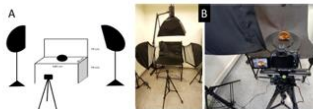
Figure 5: Schematic drawing of the photographic studio, with the dimensions indicated (5-A). Images of the studio and positioning of the structure to be photographed (5-B). Training Center for Neuroanatomy and Microsurgery.
