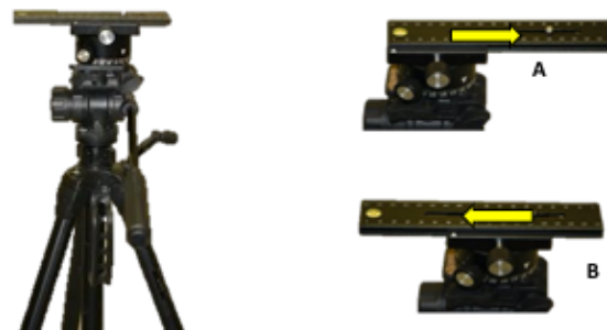
Figure 13: A: The first photo is taken focusing on the center of the structure. B: The second photo is taken focusing on the center of the structure after moving the slider 2.5 inches from the starting point.
