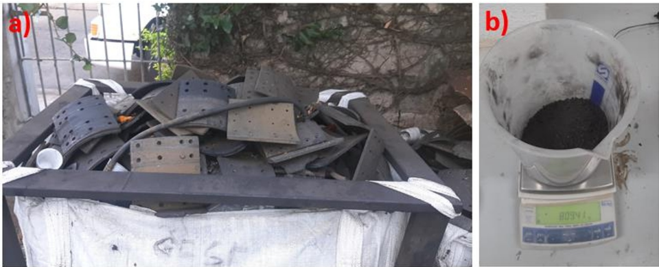
Fig. 2. Used brake lining (a) and brake lining waste grinded (b).
