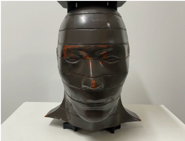
Fig. 2. Distribution of the 9 anatomical slices in the Alderson Rando phantom. Each level corresponds to the site of dosimeter insertion, as described in Table 2.
