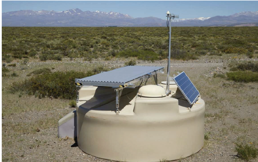
Figure 1. AugerPrime detector with the SSD atop the WCD. The UUB is hidden underneath the dome visible on top of the WCD.
