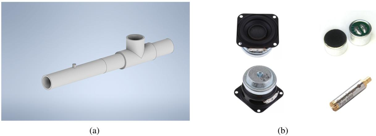
Figure C.1 – Acoustic duct to be used as an experimental platform (a) with the electroacoustic components in (b).
