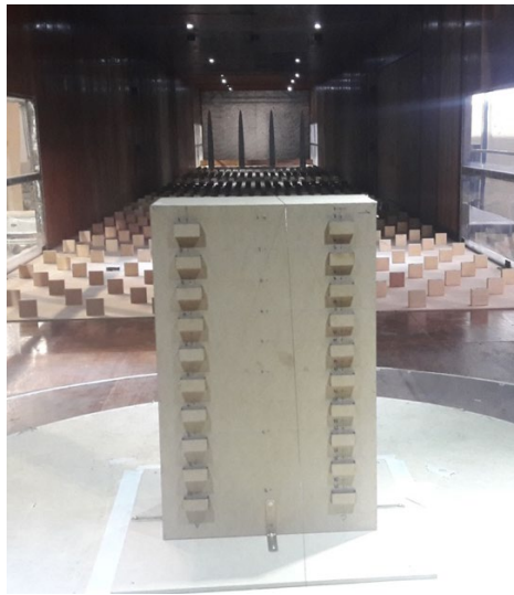
a) 1:50 scale model used in the experiment
