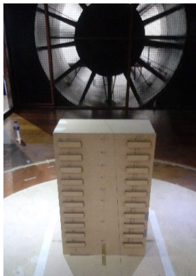
a) 1:50 scale model (isolated building)
