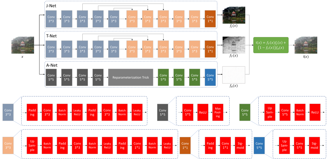
Figure 2.3: The framework of ZID. Extracted from the work developed by Li et al. [24].
