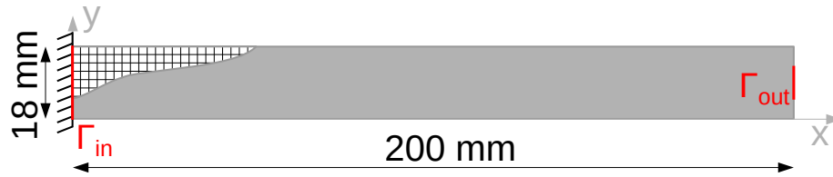
Figure 3.9 – Domain for optimization of cantilever beam with VFM.
