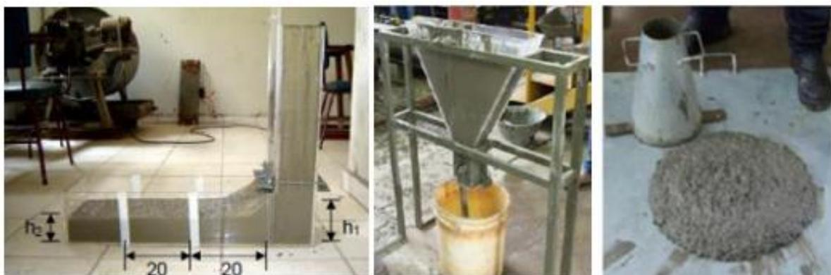
**Figura 3. 29** Ensaios *L-box*, *V-funnel* e *slump flow*.
