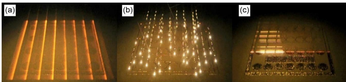
Figure 1. Preheating (a), contouring (b), and hatching (c) build sequences of an EB-PBF process [15].
