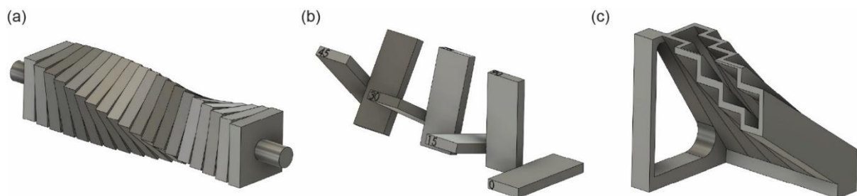
Figure 5. Different test artifacts used for surface evaluation in AM processes based on (a) Reeves [73], (b) ISO/ASTM 52903, and Galati et al. [76].
