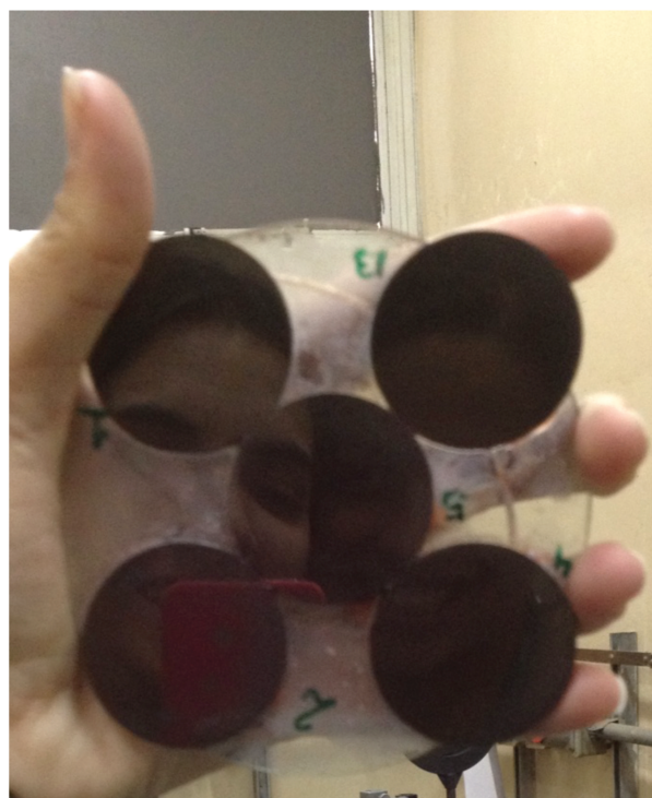
Figure 3. Blocking having 5 samples during polishing process (flat).
