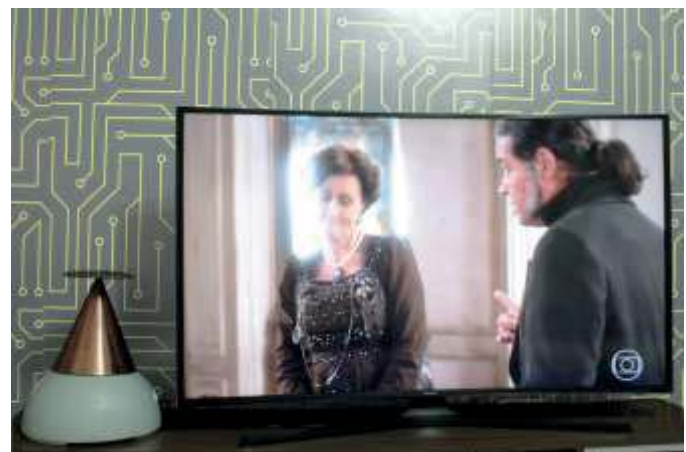
Fig. 9. A discone antenna working with a television.
