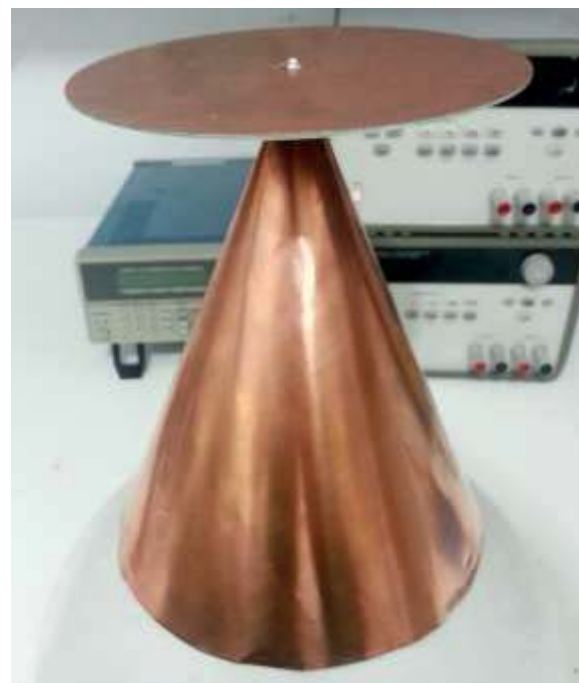
Fig. 4. Discone antenna construction.
