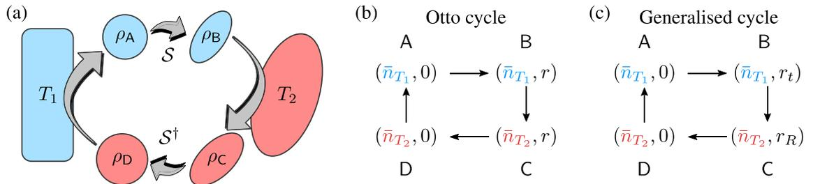
**Figure 2.** (a) Schematic diagram of the four-step protocol in which the bosonic mode is coupled with two different reservoirs. The unitaries  $S$  and  $S^\dagger$  represent the adiabatic squeezing and unsqueezing modulation of the bosonic mode. Diagrammatic representation of the (b) Otto and (c) generalised cycles. While in the former, the classicality varies during the system’s interaction with the hot reservoir, in the latter, it is kept constant.
