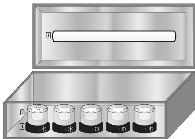
**Figure 1.** Photocatalytic bench reactor model. 1. Germicidal lamp (2,500 lux and 18.6 µW.cm<sup>-2</sup> at 254 nm); 2. Glass reactor; 3. Metal plate with immobilized TiO<sub>2</sub>; 4. Magnetic stirrer.
