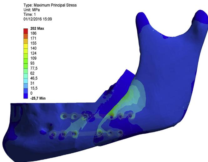
**Fig. 2.** Maximum Principal Stress values in 6-H2P group - stress dissipated to the oblique line of the mandible.
