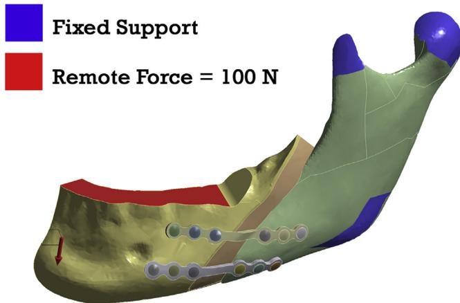
**Fig. 1.** Finite element models: locking areas (condyle, coronoid process, and insertion of masseter muscle) with 100 N loading in the midline region (arrow).
