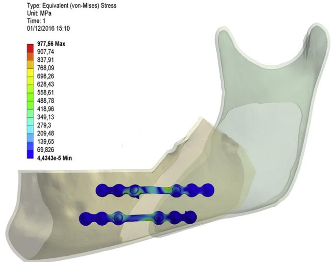
**Fig. 3.** Von-Mises Stress values in 6-H2P group - von Mises stress pattern around the top of the upper miniplate near the screw closest to the proximal segment osteotomy.
