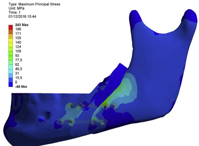
**Fig. 4.** Maximum Principal Stress values in 4-H2P group - stress dissipated to the oblique line of the mandible.
