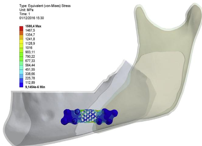
Fig. 7. Von-Mises Stress values in 3DCP group (red indicates areas of high stress concentration).
