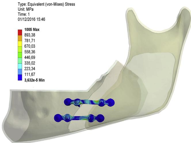
Fig. 5. Von-Mises Stress values in 4-H2P group – same characteristics of stress distribution as in the 6-H2P group.
