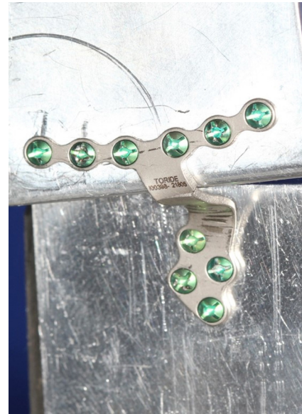
Fig. 3. Prebent plate fractured after cyclic test.
