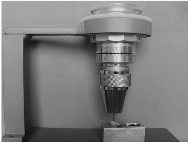
**Figure 1** Device for positioning of replica and analog torque gauge for torque insertion and detorque measurement.
