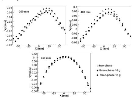
Figure 5: Axial liquid mean velocity profile Vy for: (a) air - water system, (b) air - water - FCC particles (10 g) system and (c) air -water- FCC particles (15 g) system at three different heights
