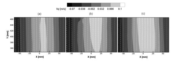
Figure 3: Vector field for liquid velocity Vy for: (a) air - water system, (b) air - water - FCC particles (10 g) system and (c) air -water- FCC particles (15 g) system at 392 mm of the injection section
