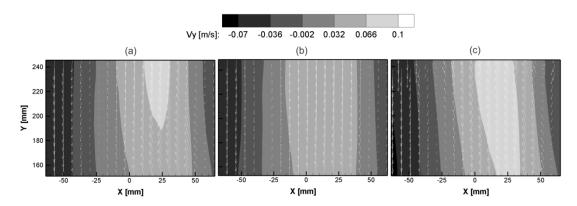
Figure 4: Vector field for liquid velocity Vy for: (a) air - water system, (b) air - water - FCC particles (10 g) system and (c) air -water- FCC particles (15 g) system at 165 mm of the injection section
