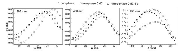
Figure 7: Axial liquid mean velocity profile Vy for: (a) air - water system, (b) air - CMC (25 % wt) c) air - CMC (25 % wt) - FCC particles (15 g) system at different heights
