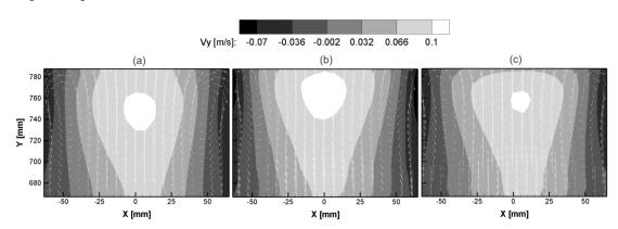
Figure 2: Vector field for liquid velocity Vy for: (a) air - water system, (b) air - water - FCC particles (10 g) system and (c) air -water- FCC particles (15 g) system at 732 mm of the injection section
