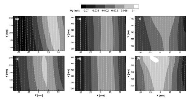
Figure 6: Vector field for liquid velocity Vy for different systems at three column heights from injection section
