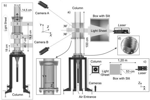
Figure 1: (a) Column, laser system, box with slit and Stereo-PIV System. (b) Fields of view (c) Details of box with slit. (d) Gas distributor
