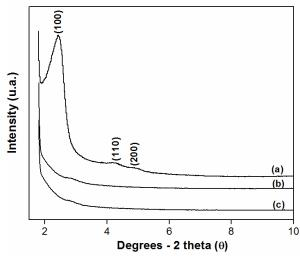
**Figure 1:** Low-angle XRD patterns of (**a**) Al-MCM-41, (**b**) 16%Ba/Al-MCM-41, (**c**) 1.4%Cr-16%Ba/Al-MCM-41.
