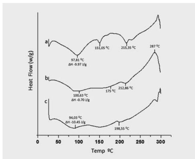
► **Fig. 3** DSC thermogram curves of (a) free bromelain, (b) hydrogel, and (c) hydrogel bromelain.
