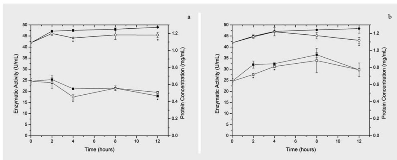
► **Fig. 1** Analysis of bromelain incorporation into hydrogel disks at (a) 4°C and (b) 25°C. Both figures show the protein concentration in control bromelain solution (●) and in the remaining solution after hydrogel immersion (○), and enzymatic activity in control (■) and remaining (□) solutions. \*Statistically significance ( $p < 0.05$ ) between control and remaining solutions. Error bars indicated the standard deviation of three replicates.
