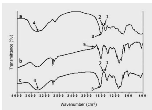
► **Fig. 4** FTIR spectra of free bromelain (a), hydrogel (b), and hydrogel with bromelain (c). The numbers 1, 2, 3, and 5 correspond to stretches at 1519  $\text{cm}^{-1}$ , 1541  $\text{cm}^{-1}$ , 1635  $\text{cm}^{-1}$ , and 1764  $\text{cm}^{-1}$ , respectively. The stretch at 3398  $\text{cm}^{-1}$  (5) in unpurified bromelain was observed at 3404  $\text{cm}^{-1}$  in the hydrogel with bromelain.
