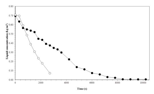
**Figure 4.** Variation in the liquid column concentration with time and gas flow rate. Experiment conditions: initial biosurfactant concentration of 0.7 kg m<sup>-3</sup> and temperature of 15 °C. Gas flow rate: ( $\bullet$ ) 3.3 × 10<sup>-7</sup> m<sup>3</sup> s<sup>-1</sup>; ( $\bigcirc$ ) 1 × 10<sup>-6</sup> m<sup>3</sup> s<sup>-1</sup>.
