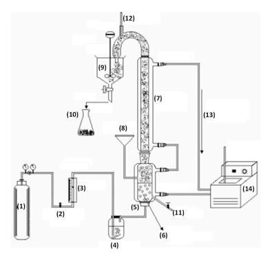
**Figure 2.** Experimental apparatus used in the fractionation of surfactin in bubble and foam column operated in a semi-bath. (1) Nitrogen cylinder; (2) Valve; (3) Rotameter; (4) Humidifier; (5) Gas distributor; (6) Liquid column; (7) Foam column; (8) Feed solution; (9) Foam breaker; (10) Sample port; (11) Sample port; (12) Thermometer; (13) Water circulation; (14) Thermostatic bath.
