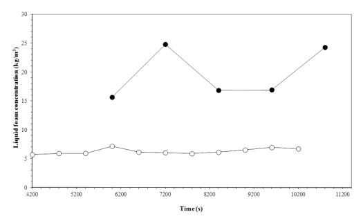
**Figure 6.** Variation in the liquid foam concentration with time and temperature. Experiment conditions: Initial biosurfactant concentration of 0.7 kg m<sup>-3</sup> and gas flow rate of  $3.3 \times 10^{-7}$  m<sup>3</sup> s<sup>-1</sup>. Temperatures:  $(\bigcirc)$  15 °C;  $(\bullet)$  35 °C.
