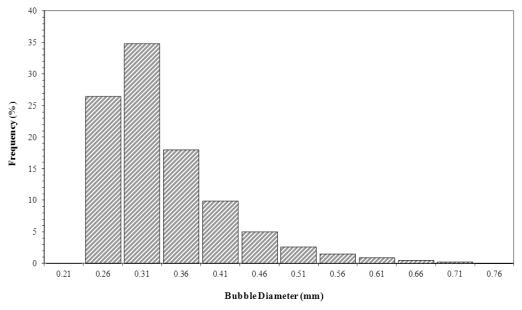
**Figure 9.** Bubble size distribution in the liquid column. Initial biosurfactant concentration of 0.7 kg m<sup>-3</sup> and gas flow rate of  $3.3 \times 10^{-7}$  m<sup>3</sup> s<sup>-1</sup>.
