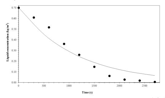
**Figure 14.** Comparison between experimental data and the model for a gas flow rate of  $1 \times 10^{-6}$  m<sup>3</sup> s<sup>-1</sup> and temperature of 35 °C.
