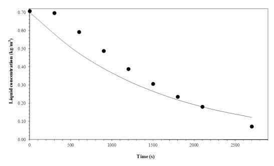
**Figure 13.** Comparison between experimental data and the model for a gas flow rate of  $1 \times 10^{-6}$  m<sup>3</sup> s<sup>-1</sup> and temperature of 15 °C.
