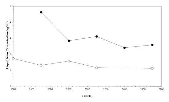
**Figure 7.** Variation in the liquid foam concentration with time and temperature. Experiment conditions: Initial biosurfactant concentration of 0.7 kg m<sup>-3</sup> and gas flow rate of  $1 \times 10^{-6}$  m<sup>3</sup> s<sup>-1</sup>. Temperatures: ( $\bigcirc$ ) 15 °C; ( $\bullet$ ) 35 °C.
