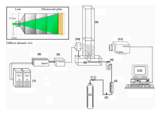
**Figure 3.** Experimental apparatus for determining the diameter distribution of gas bubbles. (1) Nitrogen cylinder; (2) Valve; (3) Rotameter; (4) Humidifier; (5) Gas distributor; (6) Column; (7) Power generation; (8) Laser source; (9) Collimator; (10) Diffuser; (11) CCD Camera; (12) Data acquisition.
