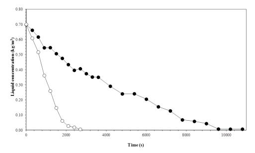
**Figure 5.** Variation in the liquid column concentration with time and gas flow rate. Experiment conditions: initial biosurfactant concentration of 0.7 kg m<sup>-3</sup> and temperature of 35 °C. Gas flow rate: ( $\bullet$ )  $3.3 \times 10^{-7}$  m<sup>3</sup> s<sup>-1</sup>; ( $\bigcirc$ )  $1 \times 10^{-6}$  m<sup>3</sup> s<sup>-1</sup>.
