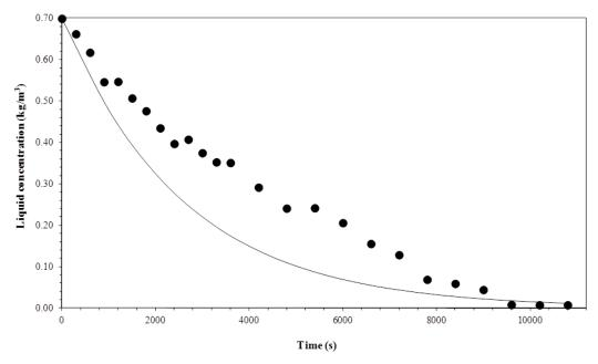
**Figure 12.** Comparison between experimental data and the model for a gas flow rate of  $3.3 \times 10^{-7}$  m<sup>3</sup> s<sup>-1</sup> and temperature of 35 °C.
