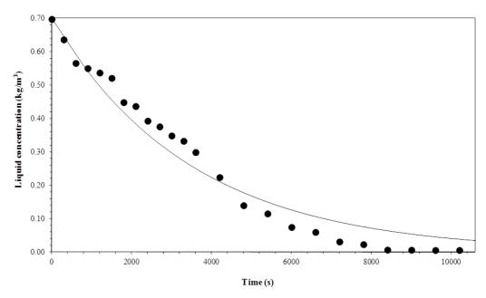
**Figure 11.** Comparison between experimental data and the model for a gas flow rate of  $3.3 \times 10^{-7}$  m<sup>3</sup> s<sup>-1</sup> and temperature of 15 °C.
