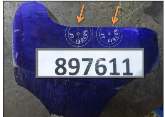
Figure 3. Location of the specimens for tests
