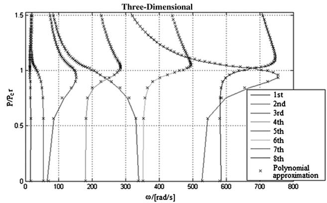
Fig. 7 Eigenfrequencies for three-dimensional vibration.
