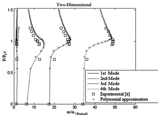
Fig. 6 Eigenfrequencies for planar vibration.
