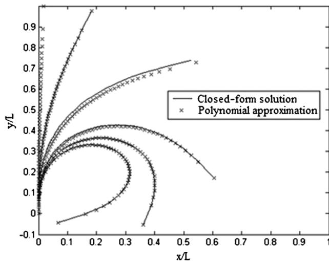
Fig. 5 Comparison of baseline deformations.
