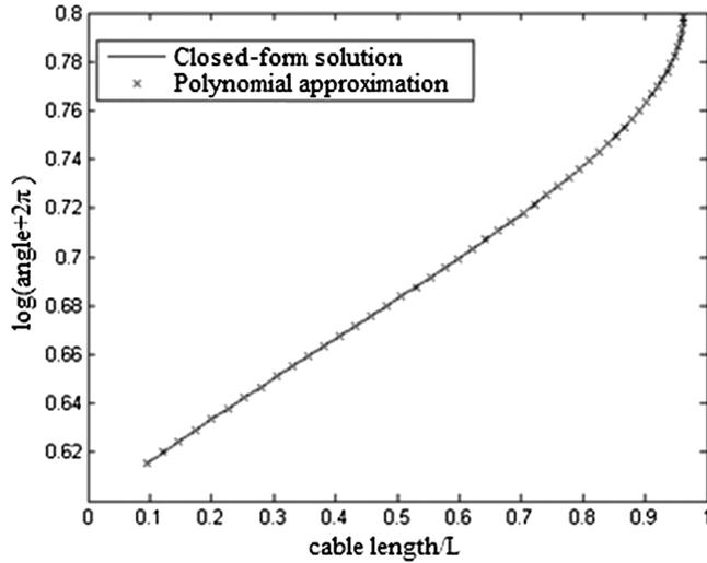
Fig. 2 Force angle  $\beta$  as a function of cable length.
