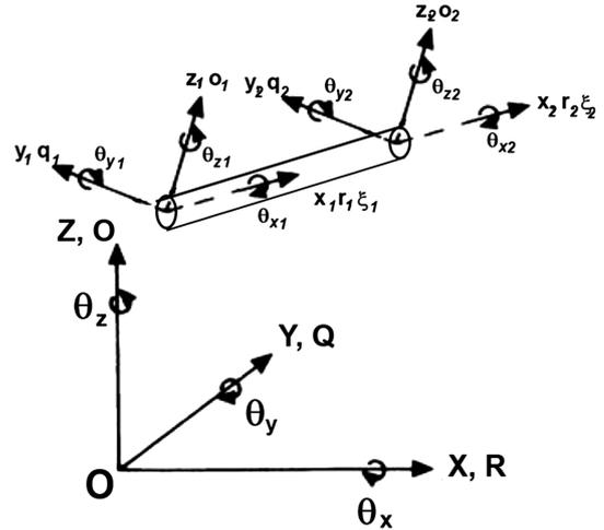
Fig. 3 Global coordinate systems and element local coordinate system.
