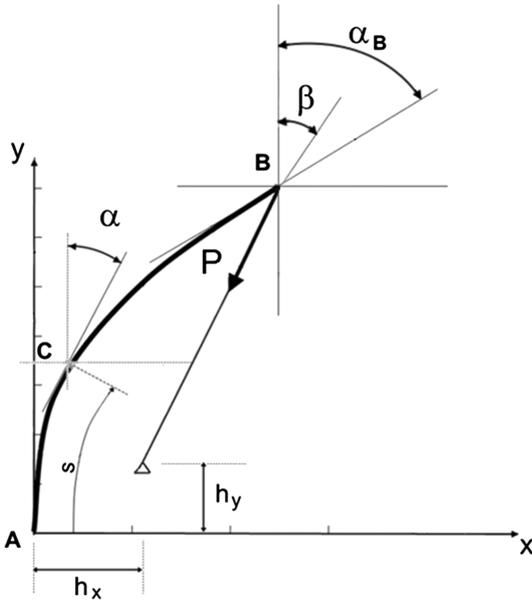
Fig. 1 Long beam pulled by an inclined cable.
