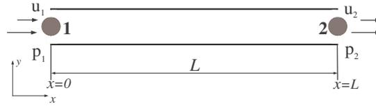
Figure 1: Two-node acoustic spectral element
