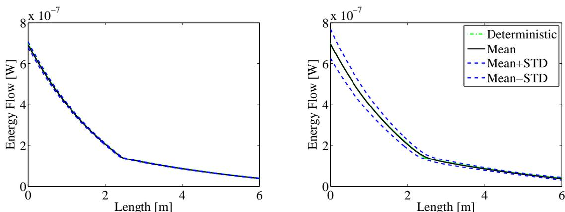
Figure 11: Flow energy for a coupling duct with COV of 2% (left-hand side) and 10%(right-hand side).
