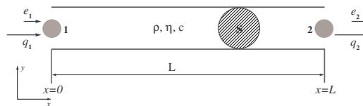
Figure 2: Two-node one-dimensional acoustic waveguide element for single duct.
