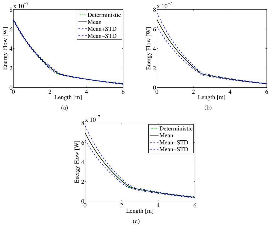
Figure 9: Mean, standard deviation and deterministic flow energy for a coupling duct with  $L$  (a),  $\rho$  (b) and both  $(L, \rho)$  (c) as random variable.
