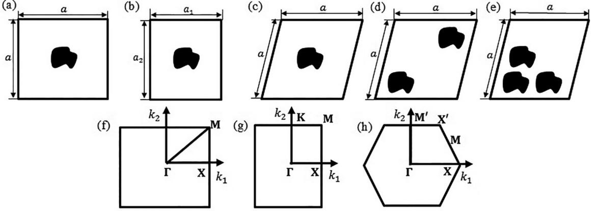
**Figure 1.** Transverse cross-section of the nano-piezoelectric phononic crystal unit cell: BaTiO<sub>3</sub> inclusions distributed in a polymeric matrix for square (a), rectangular (b), triangular (c), honeycomb (d) and Kagomé (e) lattices. First Brillouin zone for square (f), rectangular (g), triangular (h), honeycomb (h) and Kagomé (h) lattices.
