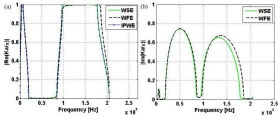
**Figure 12.** Complex elastic band structure of the real PC beam. The real part of the reduced Bloch wave vector (dimensionless) (a) calculated by WSE, WFE and IPWE methods and the imaginary part of reduced Bloch wave vector calculated by WSE and WFE methods.
