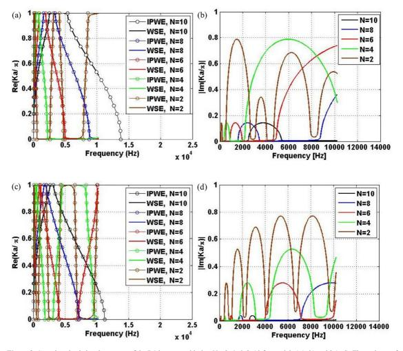
**Figure 8.** Complex elastic band structure of the PC beam considering N = 2, 4, 6, 8, 10 for models 1 (a-b) and 2 (c-d). The real part of the reduced Bloch wave vector (dimensionless) (a-c) is calculated by WSE and IPWE methods and the imaginary part of the reduced Bloch wave vector is calculated by WSE method (b-d).
