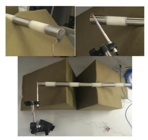
Figure 10. Experimental setup of the PC beam.
