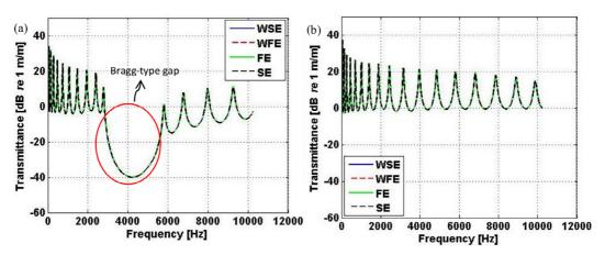
Figure 4. Transmittance of the PC beam calculated by WSE, WFE, FE and SE methods, considering models 1 (a) and 2 (b).
