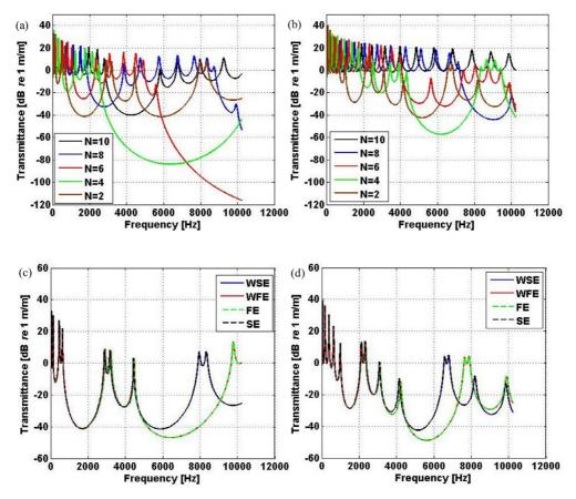
**Figure 5.** Transmittance of the PC beam calculated by WSE method for N = 2, 4, 6, 8, 10 (a-b) and the transmittance calculated by WSE, WFE, FE and SE methods for N = 2 (c-d), considering models 1 (a-c) and 2 (b-d).
