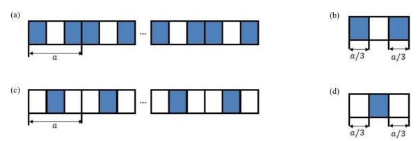
Figure 1. Schematic representation of a PC beam with N unit cells of steel (blue) and polyethylene (white) considering models 1 (a) and 2 (c). The PC beam unit cells are illustrated in (b) and (d).
