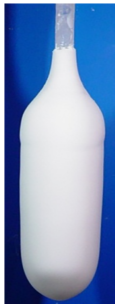
Figure 2. Green body formed by agglomerated silica nanoparticles synthesized by VAD.
