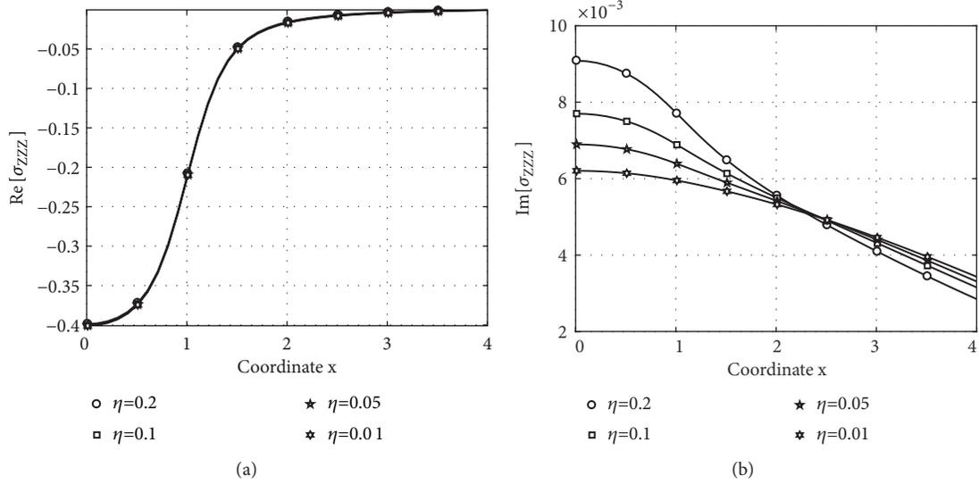
FIGURE 7: Influence of the damping factor: vertical loads.
