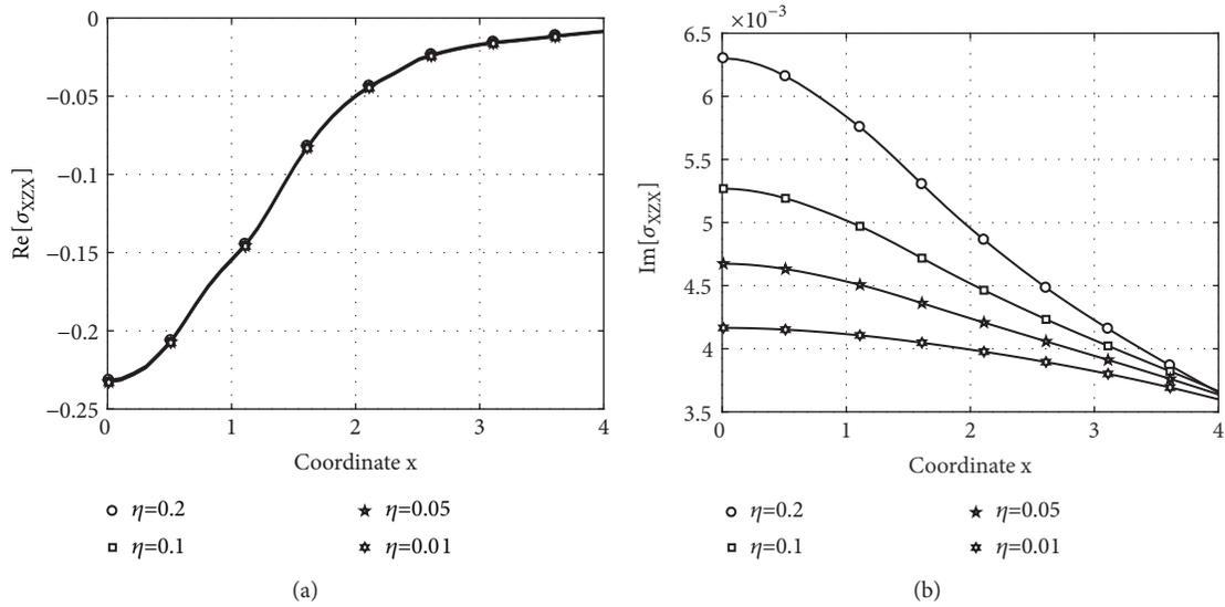
FIGURE 8: Influence of the damping factor: horizontal loads.
