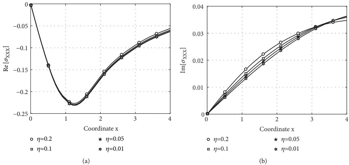
FIGURE 9: Influence of the damping factor: horizontal loads.
