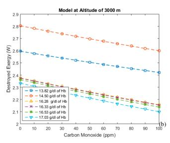
**Figure 6.** (a) Exergy efficiency and (b) destroyed exergy as functions of carbon monoxide and hemoglobin concentration at 3000 m.
