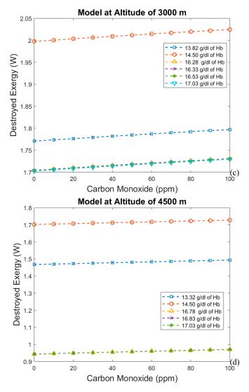
**Figure 8.** Destroyed exergy as a function of carbon monoxide and hemoglobin concentration at (**a**) 0 m, (**b**) 1500 m, (**c**) 3000 m, and (**d**) 4500 m.
