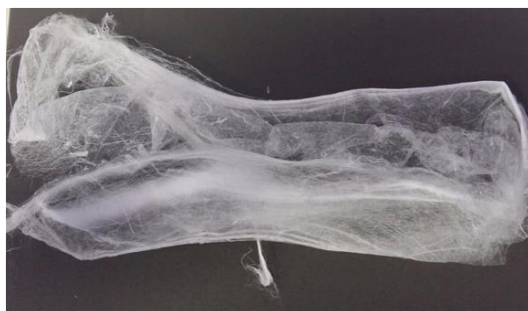
Figure 1 – Synthesized PLLA membrane obtained from rotary jet spinning process [2].
