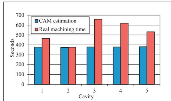
Fig.5: Machining time. Estimation from CAM and real.
