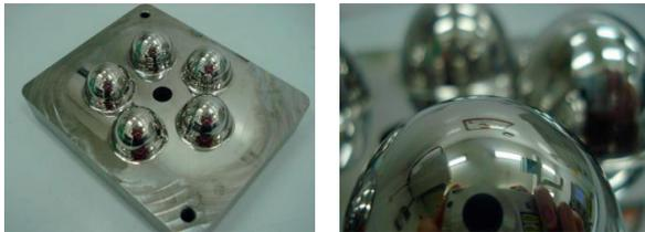
Fig. 4: Mold after polishing
