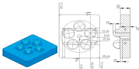
Fig. 1: Workpiece geometry.
