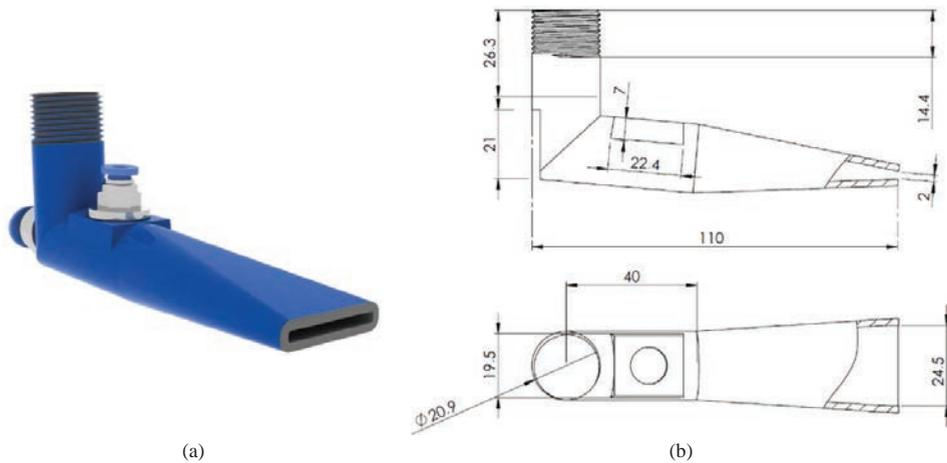
Fig. 3. (a) 3D model and (b) construction details for the designer MQL nozzle applied in the tests
