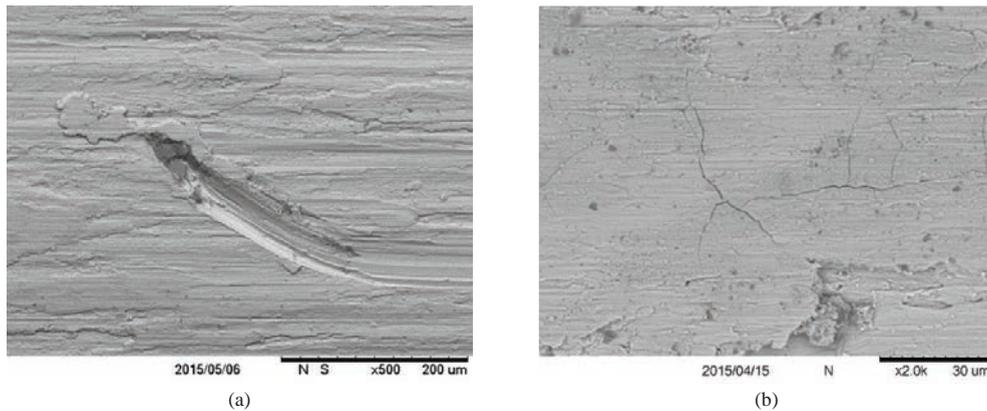
Fig. 9. (a) Embedded abrasive and (b) microcracks found on the machined surface of Ti-6Al-4V alloy after grinding with SiC wheel and MQL technique at  $a_e = 20 \mu\text{m}$ .
