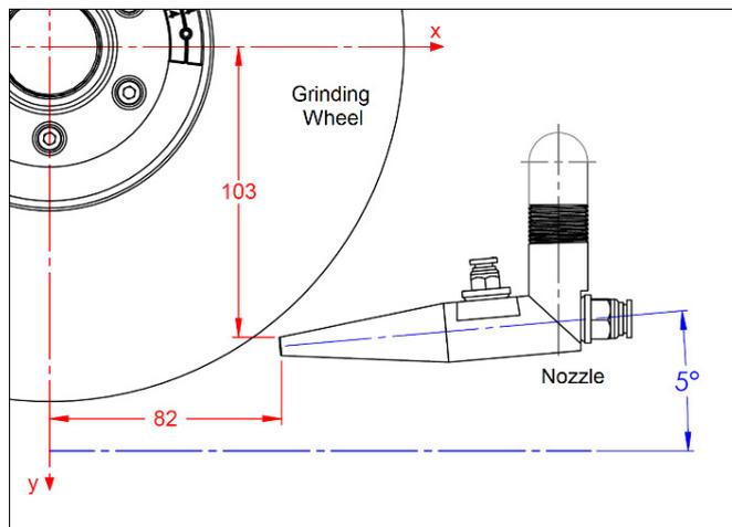
Fig. 1. Details of nozzle positioning.
