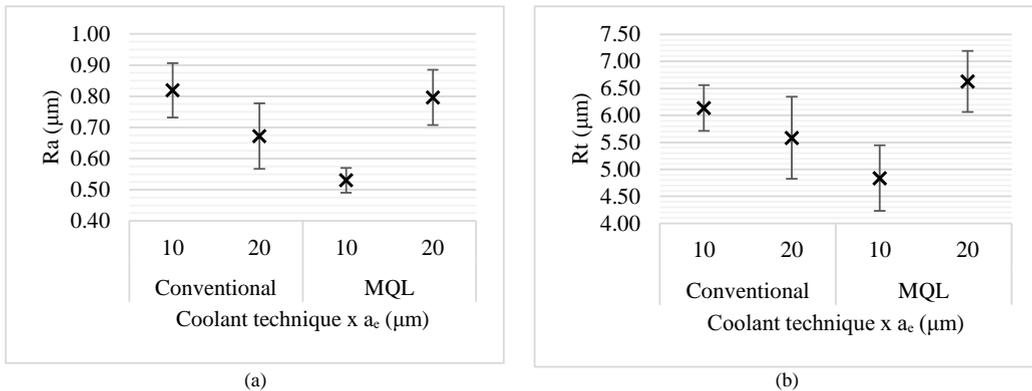
Fig. 6. Surface roughness (a) Ra and (b) Rt parameters of Ti-6Al-4V alloy after grinding with two values of depth of cut (a<sub>c</sub>) and lubri-cooling conditions as presented in the Table 1.
