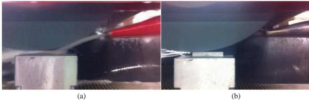
Fig. 2. Images of fluid flow and nozzle position for: (a) conventional coolant technique and (b) MQL technique.
