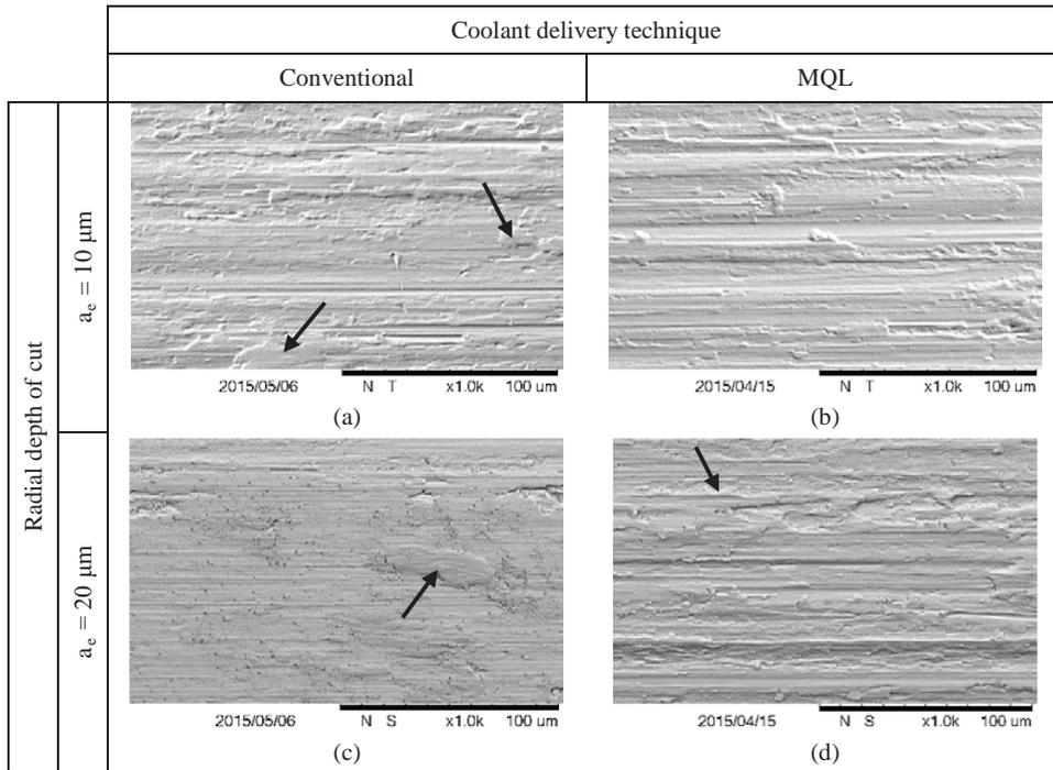
Fig. 8. SEM images of the Ti-6Al-4V alloy machined surfaces after grinding with silicon carbide wheel under different cutting conditions. The arrows indicate some points of redeposition of material on the ground surface.
