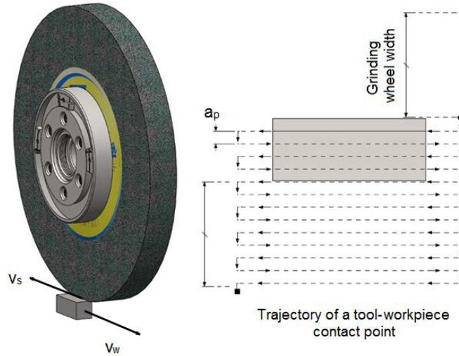
Fig. 5. Schematic of the trajectory performed by the workpiece during grinding.
