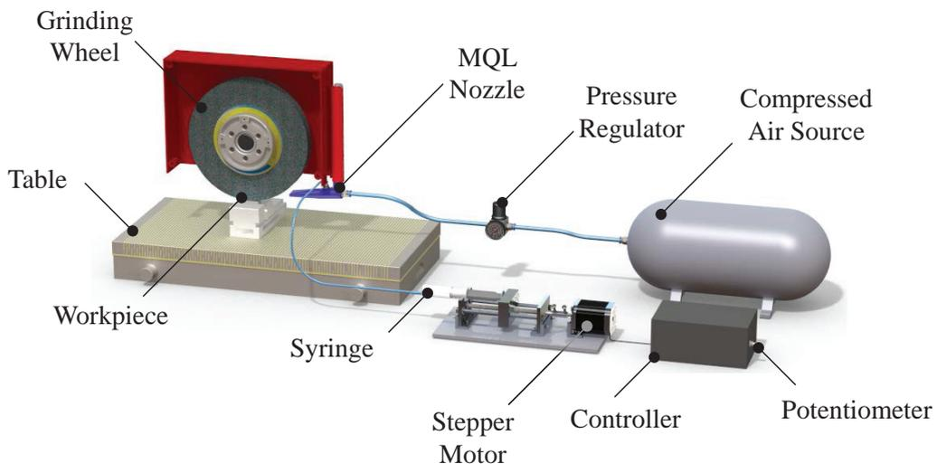
Fig. 4. Schematic of the MQL coolant system delivery.
