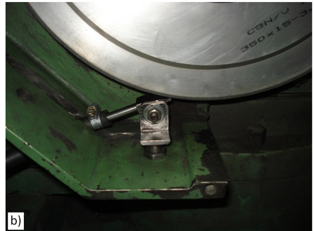
Figure 3. (a) Wheel cleaning nozzle design; (b) nozzle positioning (30° in relation to normal angle).
