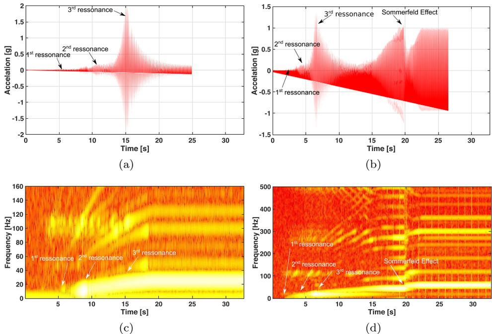
**Fig. 12** Time-frequency analysis using CWT and WPT: **a** CWT 3DOF experimental mechanical system signal without Sommerfeld effect, **b** CWT 3DOF experimental mechanical system signal with Sommerfeld effect, **c** WPT 3DOF experimental mechanical system signal without Sommerfeld effect, and **d** WPT 3DOF experimental mechanical system signal with Sommerfeld effect
