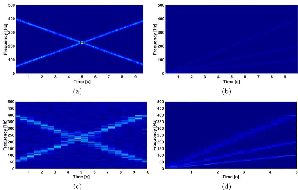
**Fig. 3** Time-frequency analysis by means of the HHT: **a** HHT of the cross chirp signal, **b** HHT of the divergent chirp signal
