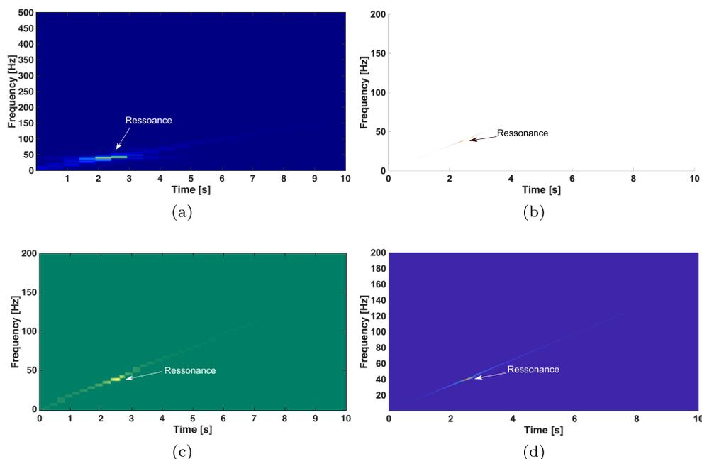
**Fig. 7** Time-frequency analysis using STFT: **a** 1DOF experimental mechanical system signal without Sommerfeld effect, **b** 1DOF experimental mechanical system signal with Sommerfeld effect, **c** STFT 1DOF experimental mechanical system signal without Sommerfeld effect, **d** STFT 1DOF experimental mechanical system signal with Sommerfeld effect
