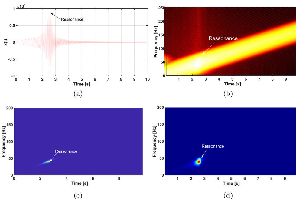
**Fig. 5** Time-frequency analysis using STFT and CWT: **a** 1DOF syntenic mechanical system signal, **b** STFT 1DOF syntenic mechanical system, **c** CWT using bump wavelet 1DOF syntenic mechanical system, **d** CWT using Meyer wavelet 1DOF syntenic mechanical
