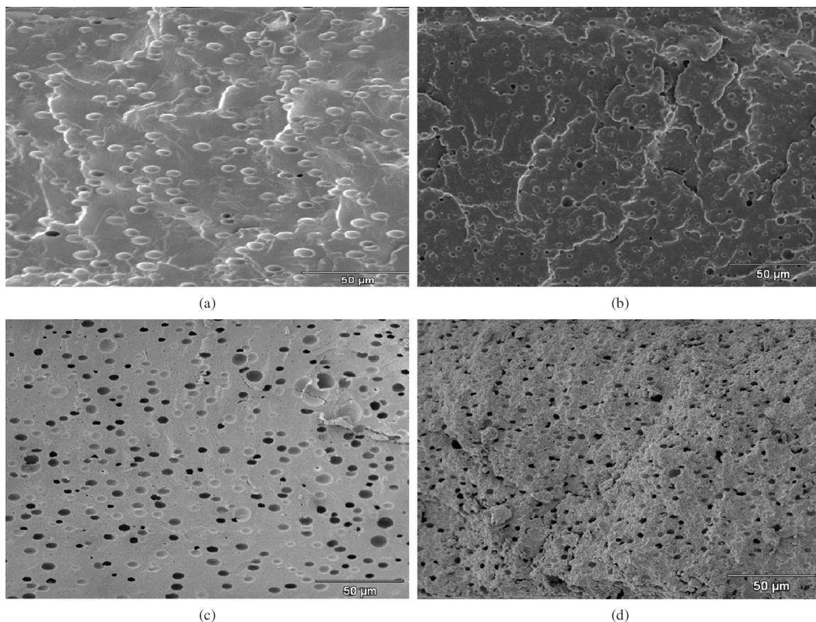
**Figure 3.** SEM micrographs of the PLDLA/PCL-T (90/10) membrane surface fracture obtained by solvent evaporation and degraded *in vitro*. a)  $t=0$  week, b)  $t=4$  weeks, c) 12 weeks, and d) 24 weeks.
