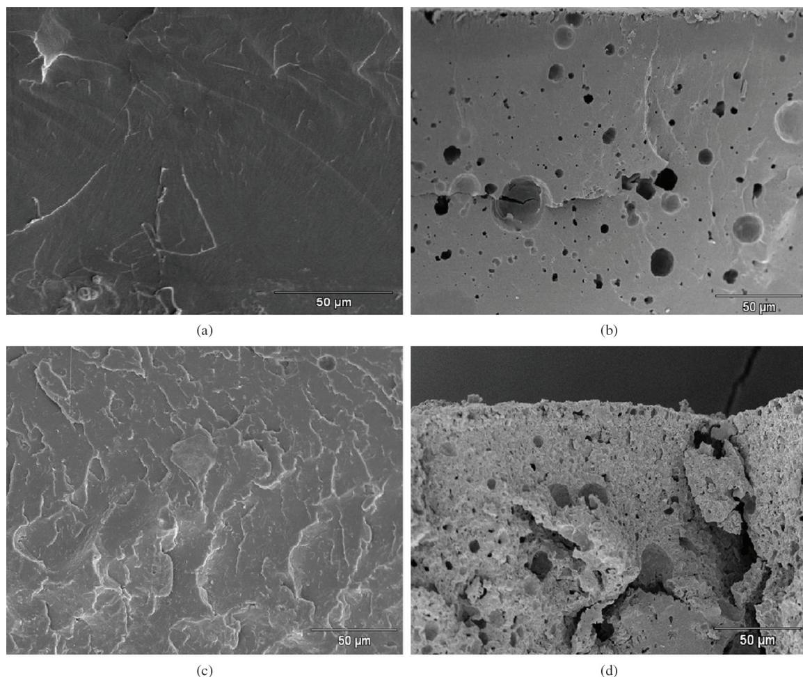
**Figure 2.** SEM micrographs of the PLDLA/PCL-T (100/0) membrane fracture obtained by solvent evaporation and *in vitro* degradation. a) t = 0 week, b) t = 4 weeks, c) t = 12 weeks, d) t = 24 weeks, 500x.
