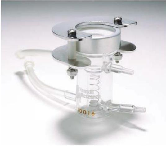
Figura 6 - Célula vertical tipo Franz. Fonte: <https://hansonresearch.com/diffusion-testing/manual-diffusion/>
