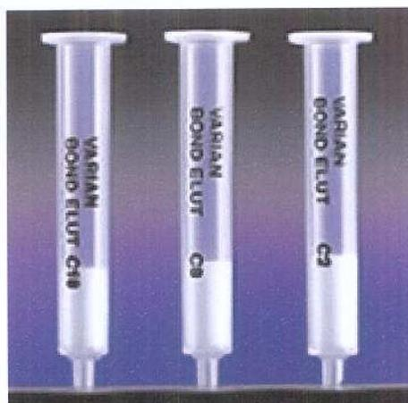
**Figura 14:** Coluna de sílica Bond Elut Jr (Varian®).
