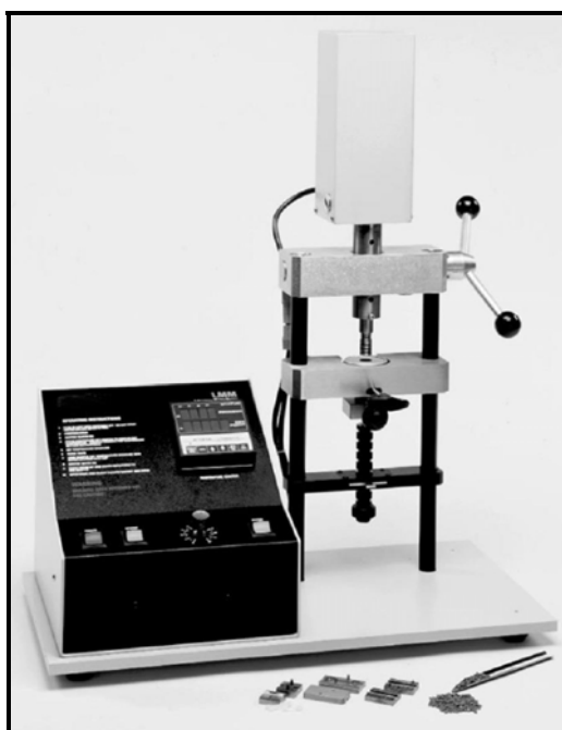
Figura 1.7. Mini-misturador LMM-Laboratory Mixing Molder (ATLAS EVALUATION PRODUCTS).
