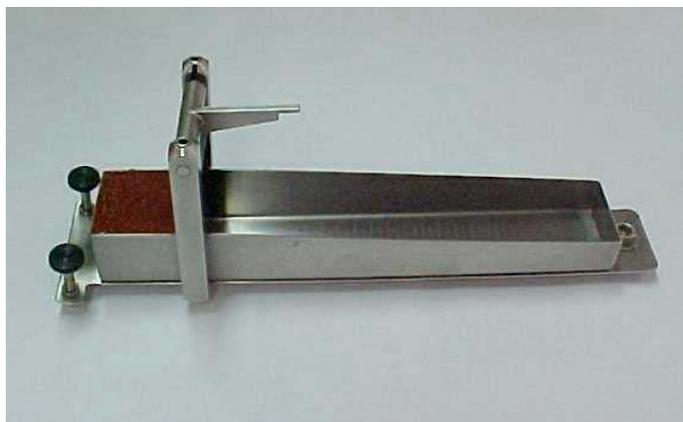
**Figura 3.1** – Consistômetro Bostwick.
