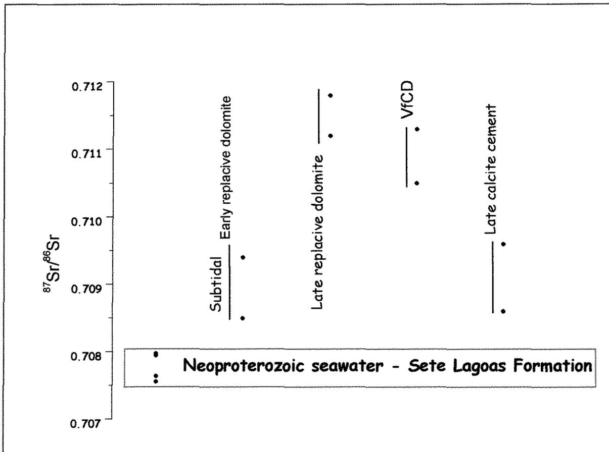
**Figure 6.6.**  $^{87}\text{Sr}/^{86}\text{Sr}$  ratios of dolomites and late calcite. The best estimated  $^{87}\text{Sr}/^{86}\text{Sr}$  ratio of Neoproterozoic seawater ranges from 0.7056 to 0.70798 according to this research.
