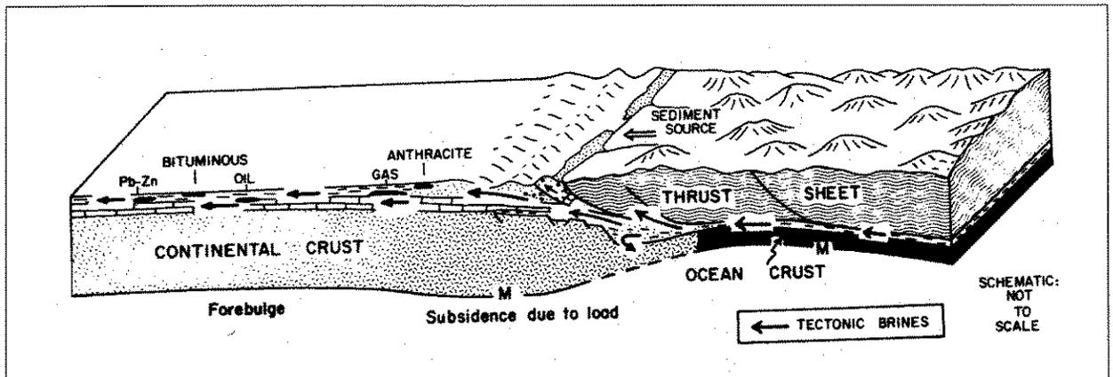
**Figure 8.1.** Block diagram of orogen when thrust sheets overrides margin sediments. Fluid flow tectonic brines are expelled from buried sediments (arrows) and injected into adjacent continent via conduit systems. These fluids may play an important role in the diagenesis of the sedimentary basin in terms of dolomitization, as well as hydrocarbon migration. Pb-Zn mineral deposits are located far from the orogenic belt. (from Oliver 1986).
