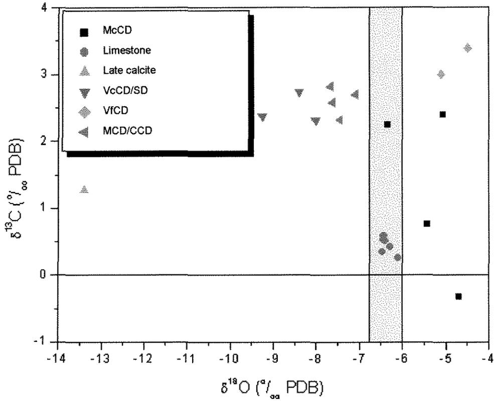
**Figure 6.5.** Cross plot of  $\delta^{18}\text{O}$  and  $\delta^{13}\text{C}$  for limestones, microcrystalline dolomite (McCD), medium to coarse crystalline dolomite (MCD/CCD), very coarse crystalline dolomite and rhombohedral saddle dolomite (VcCD/SD), very finely crystalline dolomite (VfCD) and late calcite. (The gray area represents the hypothetical seawater composition during deposition of the Sete Lagoas Formation).
