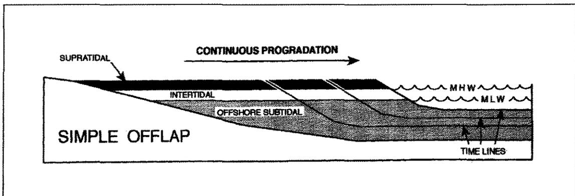
**Figure 4.16.** Tidal flat progradation: proposed model for the uppermost small shallowing-upwards successions making up the Unit 7B of the Dolomudstone member. After Pratt et al. (1992).
