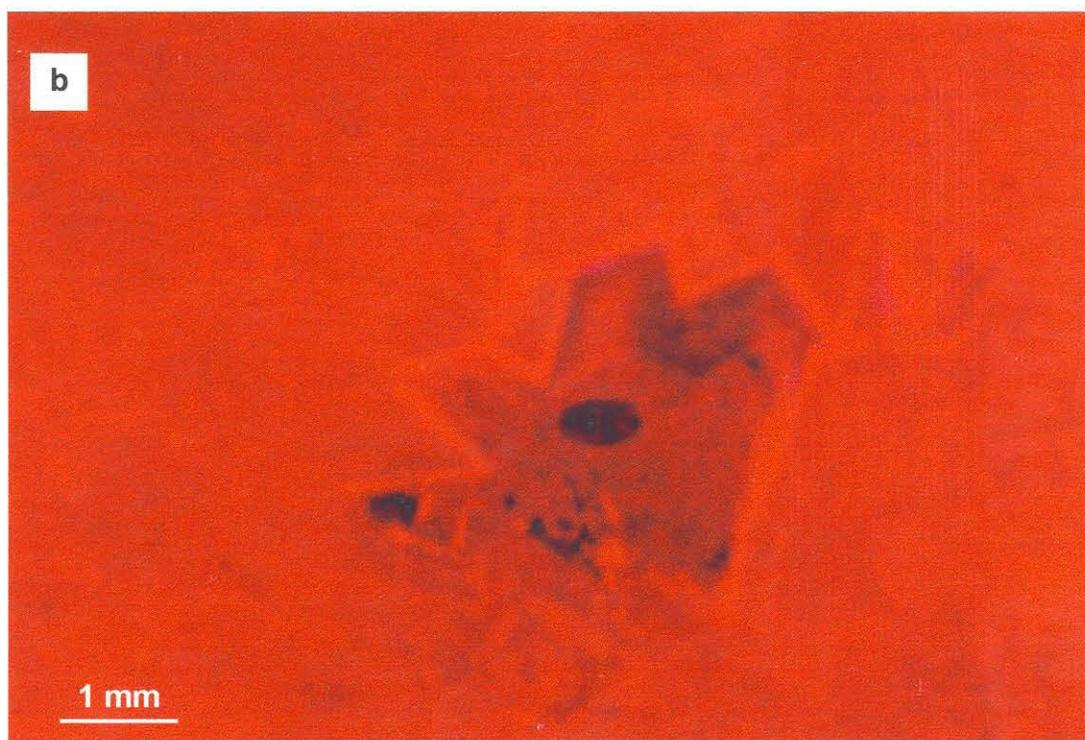
**Figure 6.3.** Dolomite cements (saddle forms) under cathodoluminescence light.
