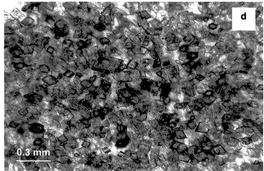
**Figure 6.4.** Petrographic features of very finely crystalline dolomite.
