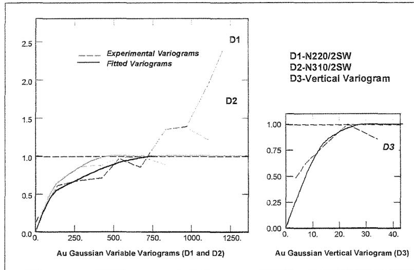
Figure 4: Variogram models for gaussian transformed Au grades
