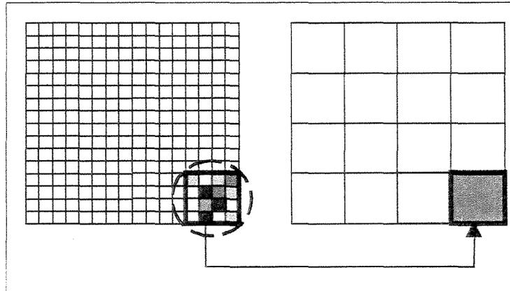
Figure 5: Selective Mining Unit (SMU) upscaling process
