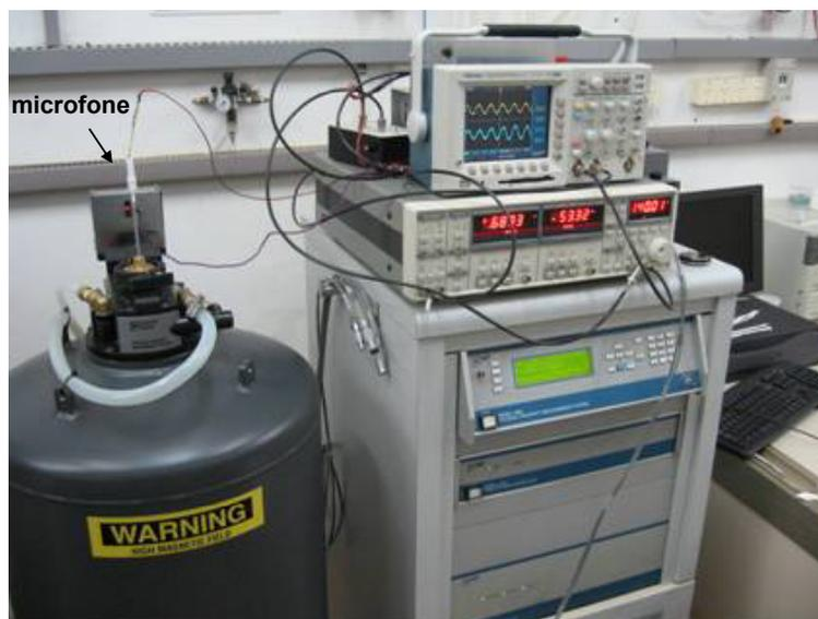
Figura 2.7: Physical Properties Measurement System (PPMS).
