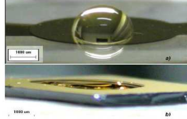
Figure 2 – Water droplets on gold surface (a), and on 3-mercaptopropionic acid (3-MPA) functionalized gold surface (b).
