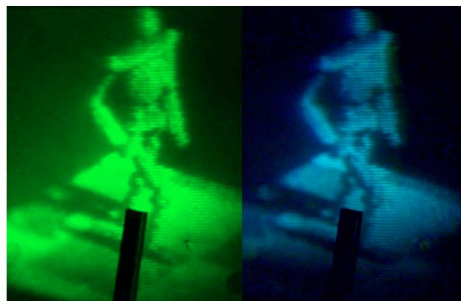
Fig. 5. (Color online) Left, the left-eye vision of the image; right, the right-eye vision of the image. The comparison between the stick and the image shows that the image is 27 cm in front of the screen.
