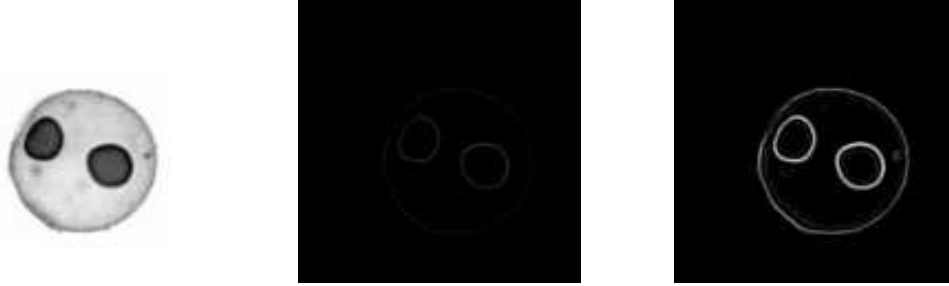
Figure 4.1: An image I (left), its Sobel gradient image \mathbf{S} I (center) and its normalized gradient image \nabla I (right).
