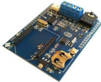
Figura 4-15: Energy Shield com Circuito Integrado ADE7753 [60]
